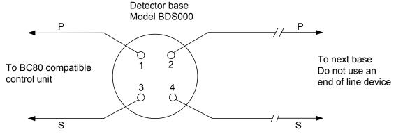
Figure 3 Wiring diagram for BDS000A
